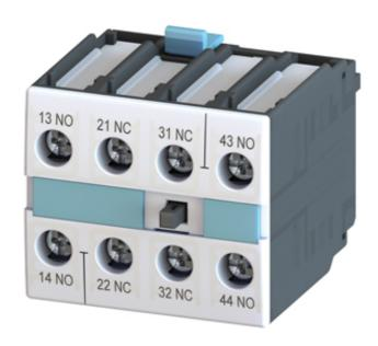
AUXILIARY SWITCH BLOCK, 22 (2NO+2NC), DIN EN50012, 4-POLE, SCREW CONNECTION, FOR MOTOR CONTACTORS, SIZE S0...S3
